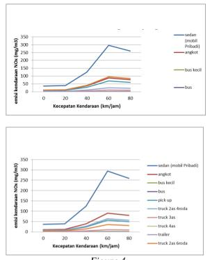
Figure 4 The number of diesel-fueled vehicle emissions in sub-urban areas
